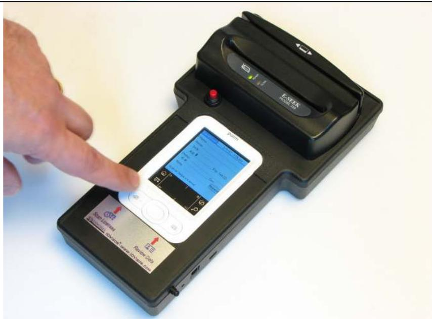
The IDvisor ID Scanner Reads 2D Bar Codes and Magnetic Stripes.
