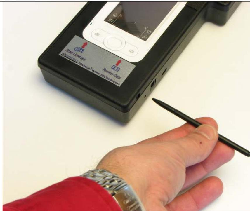
2.) Gently insert into reset hole on back of the case and Gently press Reset button.
