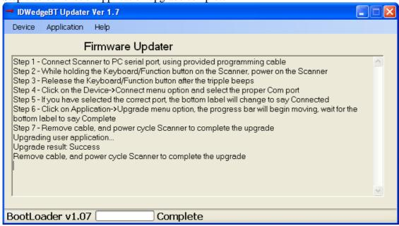
Remember to remove the cable, and power cycle the Scanner to complete the upgrade.
