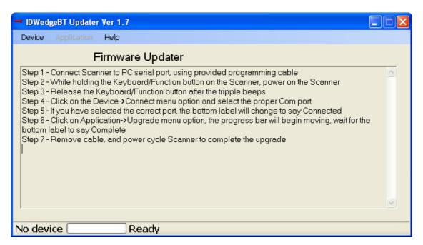
As you can see from the on screen instructions, the bottom label sends status messages, and in this case we see that no device is connected yet.
